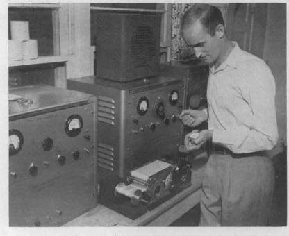
MICROBAROGRAPH OPERATOR Robert M. Yearout of Sandia Corporation's division 1633 synchronizes timing of the pen line graph which records minute changes in barometric pressure caused by TNT blast measurement shots at the Nevada Test Site. The equipment is located in Las Vegas, more than 60 miles southeast of the testing area.
